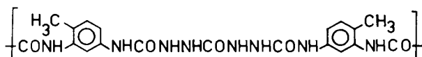
Figure 7. Molecular structure of soft and hard segment of photochromic polyester urethane with partly photochromic soft segments.
