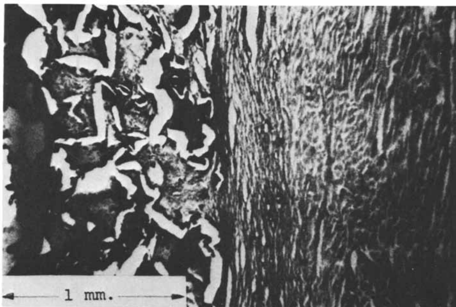
Figure 7. Histological section showing vigorous tissue ingrowth into coarsest porous polyurethane (150–250 \mu\text{m} pores).
